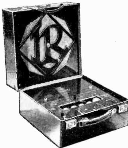
The new Langham portable set, with mechanical wave-change arrangement.
