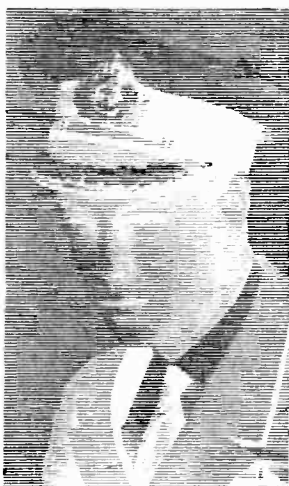
The black lines of the negative image represent the insulating gum deposit on the copper foil as used in the Fultograph system. The picture is formed at the receiver by the interrupted currents of varying duration being applied to a moistened paper sensitive by colouration to the passage of current.
