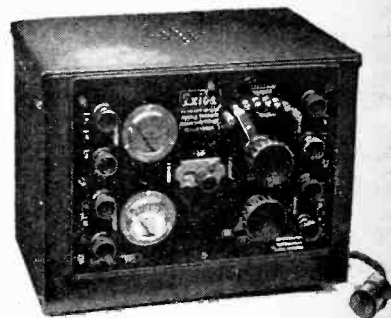
Exide combined H.T. and L.T. trickle charger with meters for checking charging rates. By means of a special switch the mains are never connected to the receiver.
