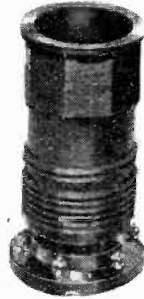
The Formo two-range tuner, with reaction winding between long- and short-wave coils.
