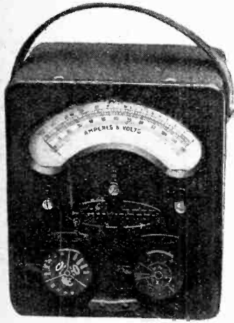
The Avometer, a universal testing instrument.
