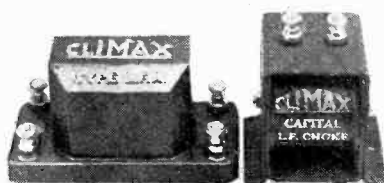
Climax Capital L.F. choke (right) and L.F.A. transformer.
