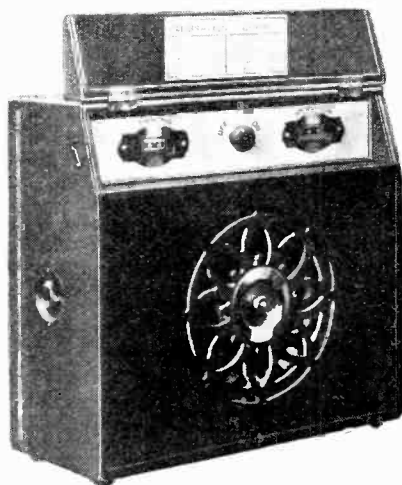
A new portable. The Marconiphone self-contained receiver with edgewise scale tuning dials.
