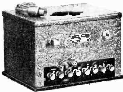
Met-Vick combined eliminator for H.T., L.T., and grid bias. The series anode feed resistance method and a full-wave rectifier is incorporated.
